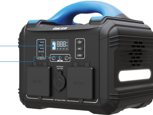
(2) You can charge the unit through the USB-C PD port at the same time, which enables it to reach full charge faster. When charging through USB-C PD and DC ports simultaneously, the IN and PD indicators, and the 5-bar battery power meter, flash on the LCD display. When the unit is fully charged, the battery meter is always on.
